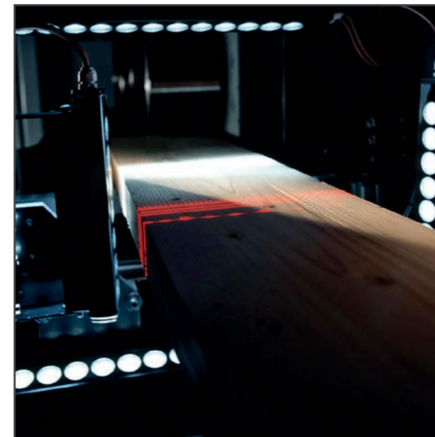
► The Multi-Sensor scanning technology scans workpieces for best wood utilization.
