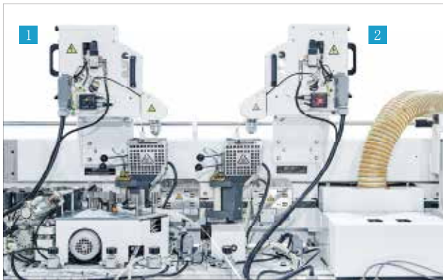
Gluing unit and pre-melter: Quick-change application unit with hot melt glue supply from top. On-demand availability and perfect glue quality with Quickmelt. (1 # optional PUR coating)
