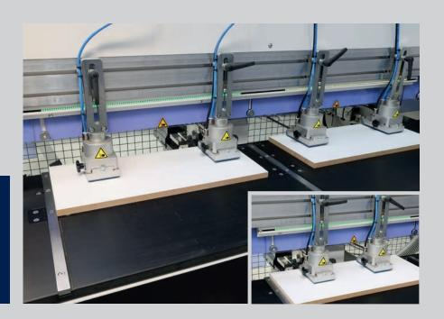
**OPTICAL LED ASSISTANCE SYSTEM** to assist the machine operator in the processing of workpieces. The LED bar lights in the areas where the workpieces are to be positioned. The length of the illuminated areas corresponds to the length of the workpieces to be positioned. Once the positioning is correct, the color of the LED bar changes.
