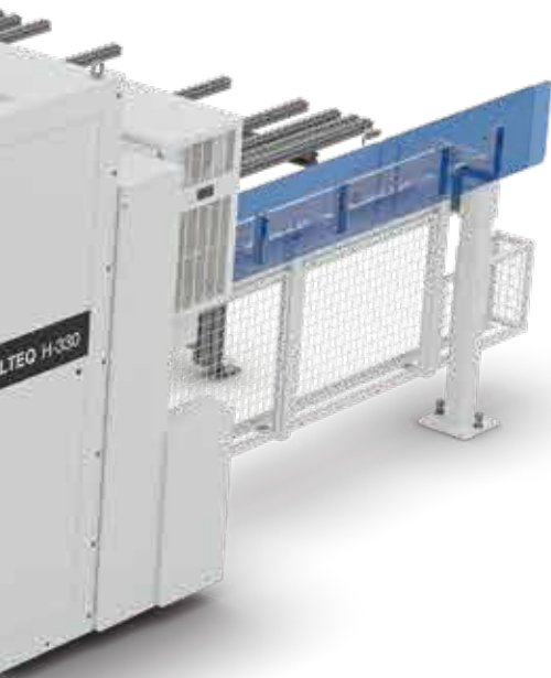
The lower safety fence prevents entry into the working area.
