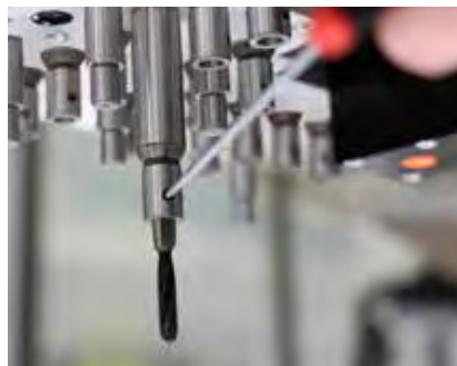
Weldon change system for a drill change with tools
