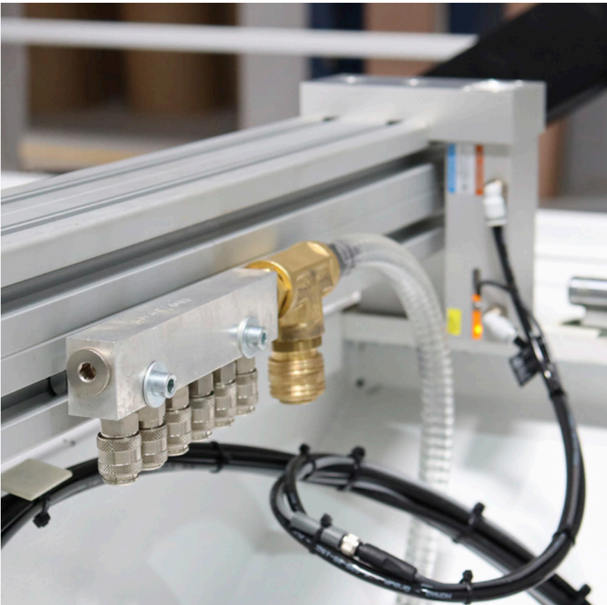
Option: Vacuum connections ▪ E.g. for templates and clamp type multi clamps
