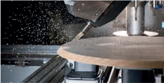
Chamfer trimming on a table top
