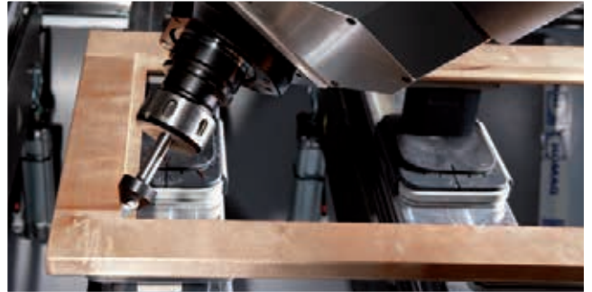
Square corner routing for a glass rebate
