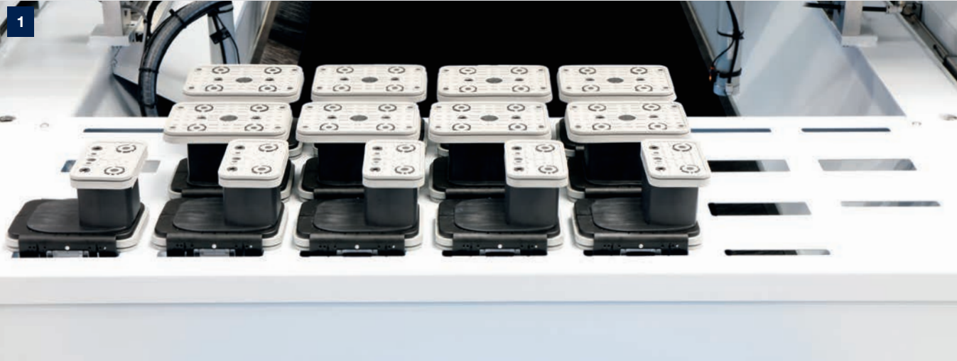
Suction cup storage area Storage area laterally integrated into the machine for vacuum suction cups for easy and fast access
