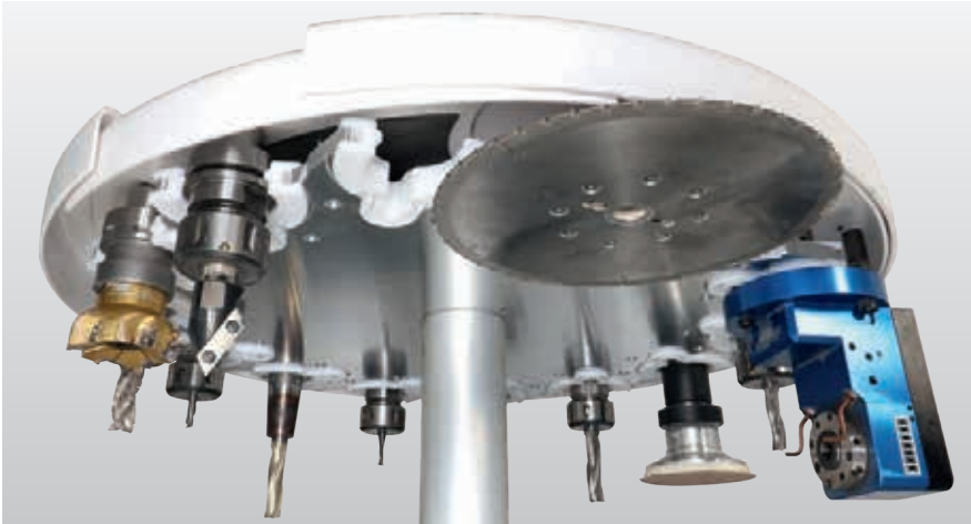
14-fold tool changer moving in X-direction
