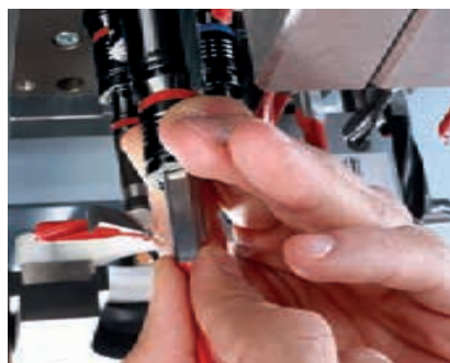
Patented quick-change system for a drill change without tools to reduce setup times.
